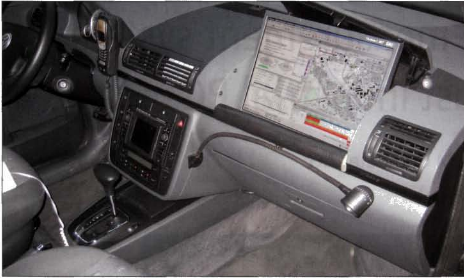
Figure 2. The mobile wireless measurement system with mobile wireless devices made by various manufacturers in a vehicle of the O 2 network operator.
