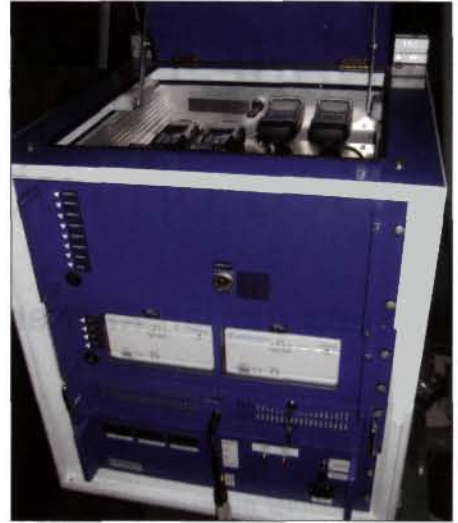
Figure 3. The display installed in the vehicle provides a fast overview of the location-dependent transmitter power.
